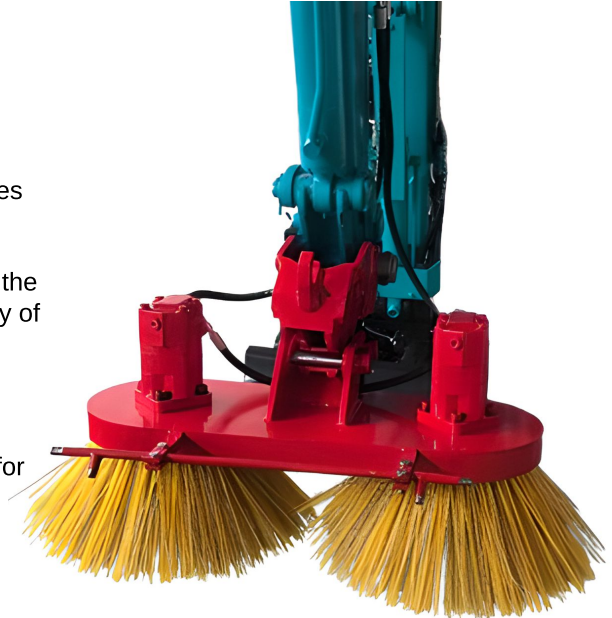
Twin Motor/Twin Brush Hydraulic Sweeper
